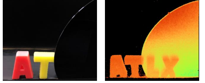
Fig. 4. RGB image (left) and depth image under 1310 nm wavelength illumination (right).
